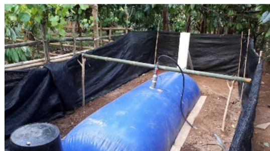
Figure 3B: Balloon/bag digester. Source: Marco Ghiandelli, “Development and Implementation of Small-scale biogas balloon biodigester in Bali, Indonesia.” (KTH Industrail Engineering and Management, 2017).
