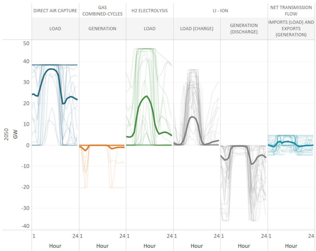
Figure 20 Electricity balancing from key technologies in ERCOT in 2050 in the 350 – Low Land NETS case
