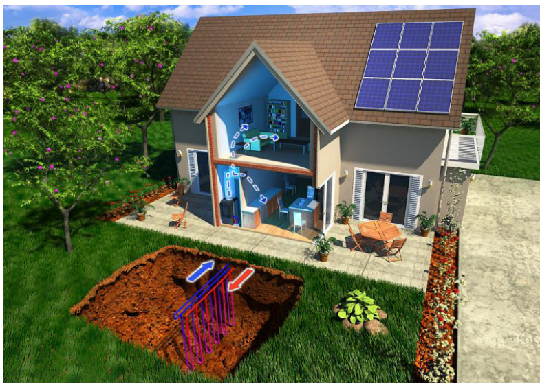
Figure 4.2.7. Geothermal heat pump piping and rooftop photovoltaic array in Whisper Valley community (Whisper Valley, 2020).
